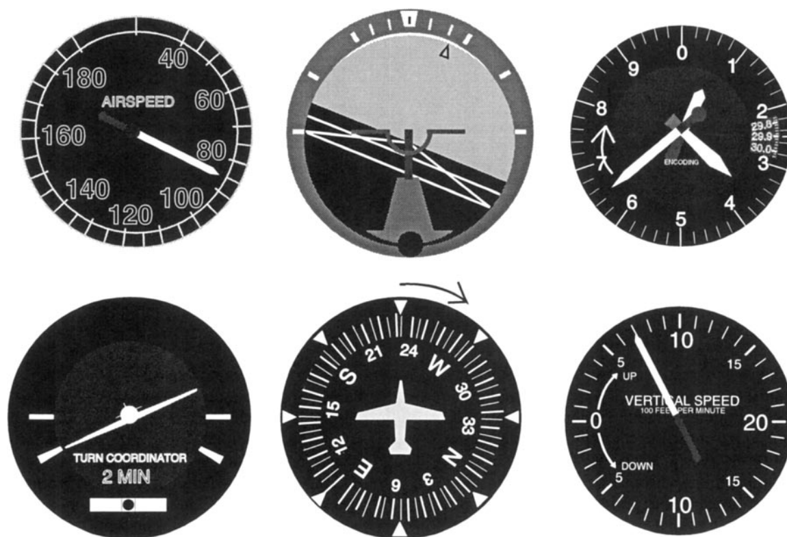
Figure 1. Example Display (climbing turn) from the Instrument Relationships PLM. Motion of needles or outer dials is depicted by arrows inside or outside the dials respectively.
